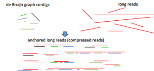
Figure 1a | Map de Bruijn graph contigs to the long reads. The long reads are in red, the de Bruijn graph contigs are in other colors. Each long read is converted into an ordered list of contigs, termed compressed reads.
