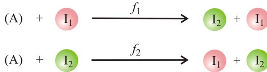
$$\frac{dx_1}{dt} = f_2 x_2 \quad \text{and} \quad \frac{dx_2}{dt} = f_1 x_1$$
