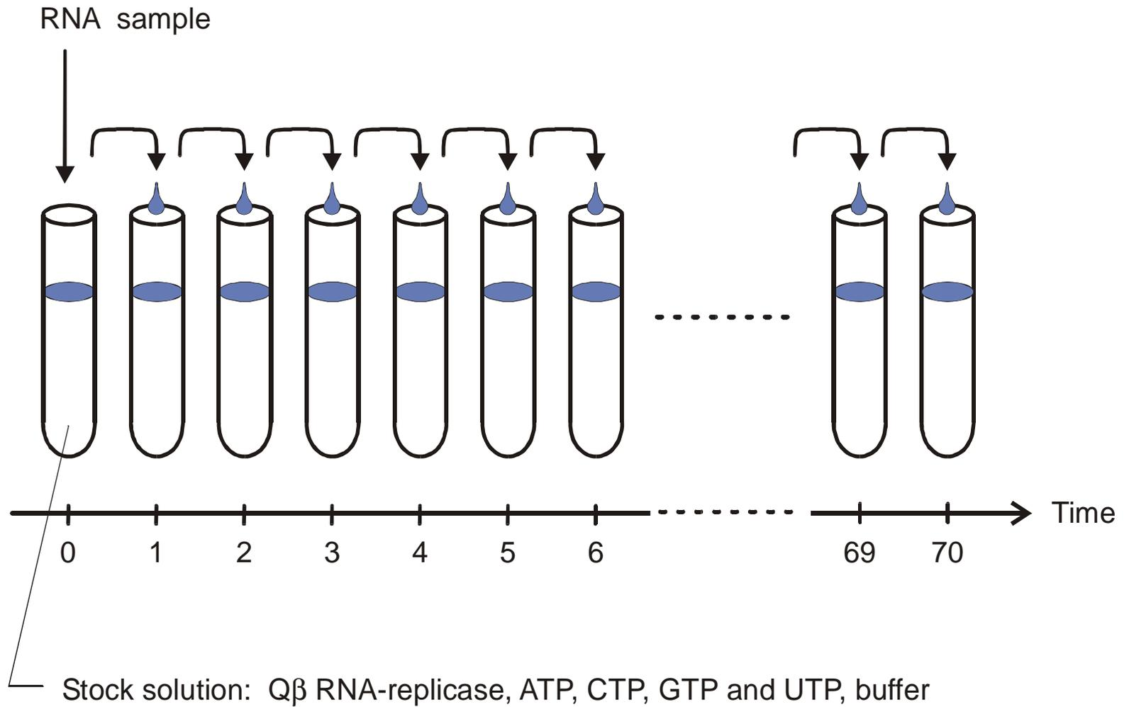
Application of the serial transfer technique to RNA evolution in the test tube
