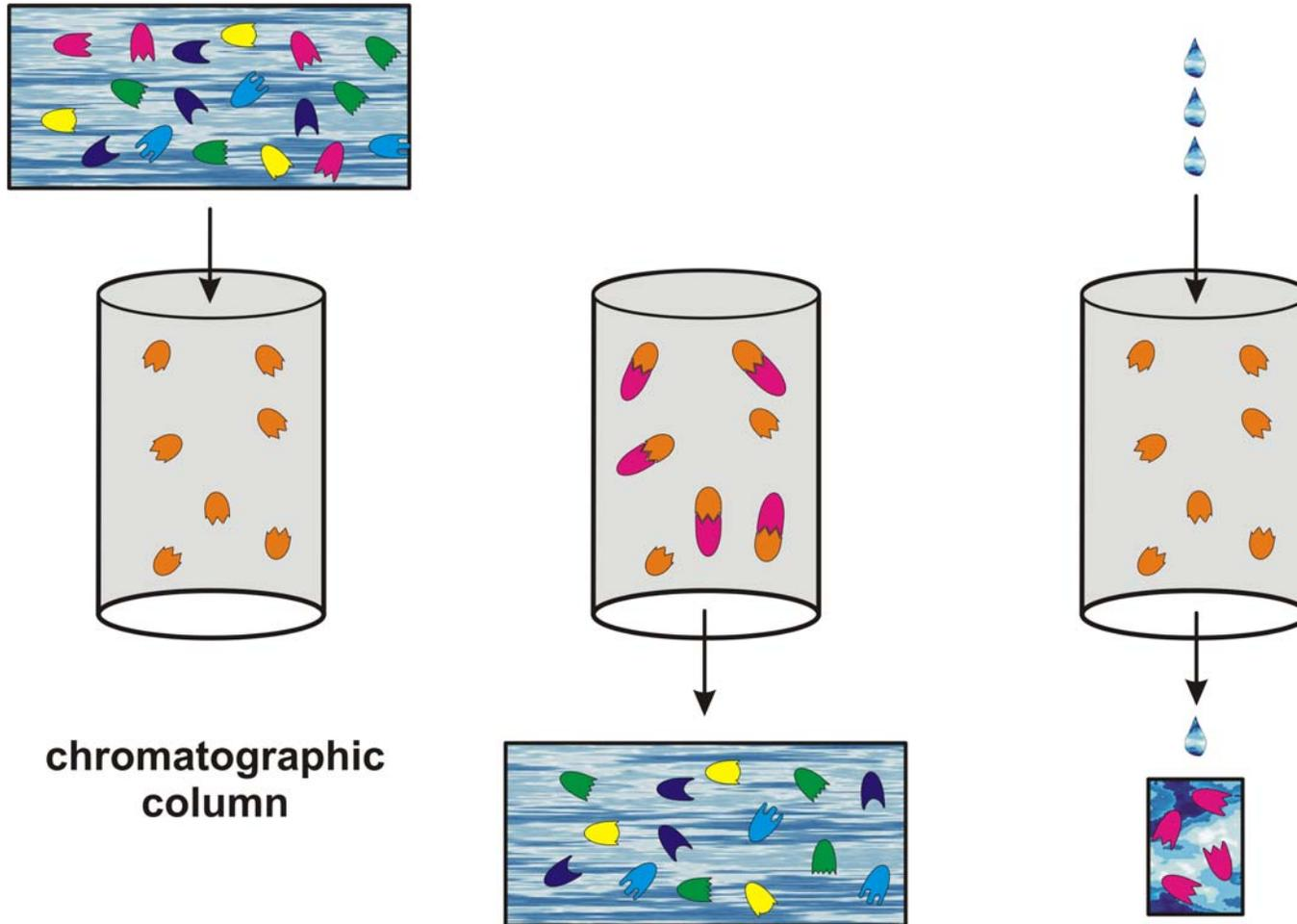
The SELEX-technique for evolutionary design of strongly binding molecules called aptamers
