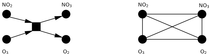
Figure 4: Representations of the reaction \text{NO}_2 + \text{O}_3 \rightarrow \text{NO}_3 + \text{O}_2 in hypergraph form drawn as the equivalent directed bipartite graph (l.h.s) and as part of a substrate graph (r.h.s).
