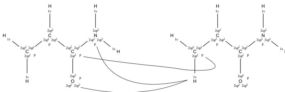
**Fig. 2.** Selected allowed interactions between two propenamide molecules. The molecules are shown with their atoms surrounded by their valence orbitals. Curved lines indicate some of the allowed interactions:  $p$ - $p$ ,  $p$ - $s$ , and  $p$ - $l$  (the  $sp^2$  orbital on O is occupied by a lone pair and thus a  $l$ -type orbital).
