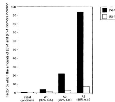
FIG 1. Asymmetric autocatalysis of chiral pyrimidyl alkanol (**1**). Runs A1–3 correspond to Table 1. The enantiomeric excess of (S)-**1** increases from 5 to 89% e.e. without the use of additional chiral auxiliaries. During the reactions (runs A1–3), the (S)-**1** increases by a factor of 94 times, while (R)-**1** increases by a factor of only eight times.
